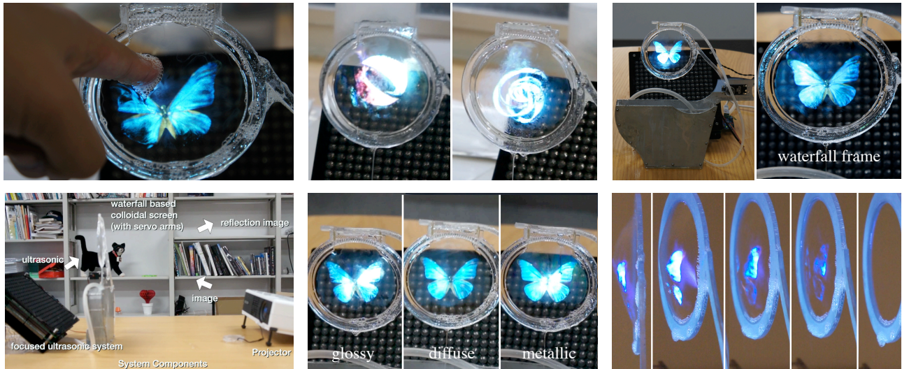
Figure 1: (top-left)flexible screen. (top-center)Omnidirectional display. (top-right)waterfall frame. (bottom-left) system overview. (bottom-center) reflective material display. (bottom-right) deformable display
